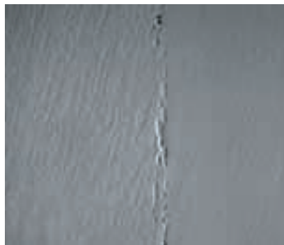
Figure 3 - SEM at 150X magnification displays the mechanical interlock in the hexagonal engagement area between the flats of the implant and abutment.
